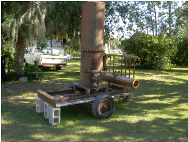
Photo 1 - Farmers looking for ways to produce power without petroleum might benefit from gasification systems, which use wood as fuel. These systems require a device called a down-draft wood gas generator, like the one pictured here. There will be a live demonstration of gasification at the first Florida Small Farms and Alternative Enterprises Conference in Kissimmee, Aug. 1-2. Photo by Clay Olson
